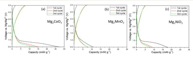
Fig. 3 Electrochemistry of Mg-rich disordered rocksalts. Charge/discharge profiles of the first three cycles of (a) Mg<sub>2</sub>CoO<sub>3</sub>, (b) Mg<sub>2</sub>MnO<sub>3</sub>, and (c) Mg<sub>2</sub>NiO<sub>3</sub> in Mg cells at 60 °C using 0.3 M Mg[B(hfip)<sub>4</sub>]<sub>2</sub> in DME as the electrolyte at a current density of 10 mA g<sup>-1</sup>.
