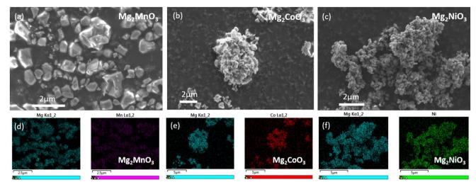
Fig. 2 Particle morphology and uniform elemental distribution. SEM and EDX of the  $Mg_2TMO_3$  samples. SEM images of (a)  $Mg_2MnO_3$ , (b)  $Mg_2CoO_3$ , and (c)  $Mg_2NiO_3$  showing primary particle sizes from 0.1 to 1  $\mu$ m. EDX elemental mapping of (d)  $Mg_2MnO_3$ , (e)  $Mg_2CoO_3$ , and (f)  $Mg_2NiO_3$ , which shows homogeneous distribution of elements in the samples.
