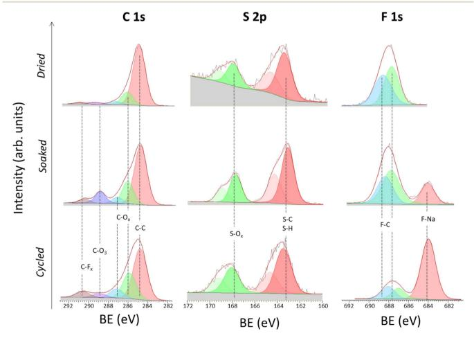
Fig. 5 Ex situ C 1s, S 2p, and F 1s XPS spectra of the surface of the NaSTFSI-co-PET-MP/4A membrane (dried), incorporating EC: DMC: FEC molecular transporters (soaked) and after cycling for 5 cycles in a Na|Na symmetric cell under 10  $\mu$ A cm<sup>-2</sup> (cycled).
