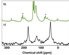
Fig. 2 (a) FT-IR spectra of NaSTFSI, PET4A, PETMP, and NaSTFSI-co-PET-MP/4A membrane.  $^{1}H \rightarrow ^{13}C$  CPMAS NMR spectrum of (b) NaSTFSI and (c) NaSTFSI-co-PET-MP/4A electrolyte, recorded at 10 kHz and 14.1 T. Note: Signals marked with asterisks (\*) are spinning side-bands.
