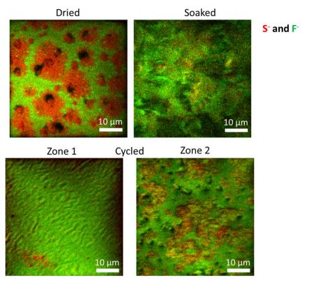
Fig. 6 ToF-SIMS combined mappings of S<sup>-</sup> (red) and F<sup>-</sup> (green) ionic fragments on the surface of the NaSTFSI-co-PET-MP/4A membrane (dried), incorporating EC: DMC: FEC molecular transporters (soaked) and after cycling for 5 cycles in a Na|Na symmetric cell under 10  $\mu$ A cm<sup>-2</sup> (cycled).
