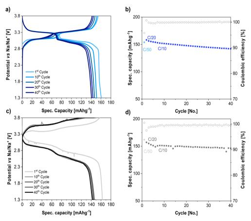
Fig. 7 Voltage profile and cycling performance of PW cathode using (a and b) 1 M NaPF<sub>6</sub> in EC: DEC (3:7 vol%) liquid electrolyte and (c and d) NaSTFSI-co-PET-MP/4A electrolyte at 40 °C.
