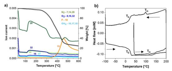
Fig. 3 (a) TGA/MS and (b) DSC of the NaSTFSI-co-PET-MP/4A membrane.
