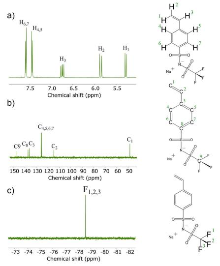
Fig. 1 (a) <sup>1</sup>H, (b) <sup>13</sup>C, and (c) <sup>19</sup>F-NMR spectra and structure of NaSTFSI sodium salt monomer.
