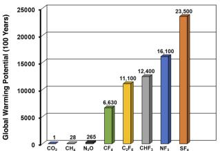
Fig. 1 One hundred year global warming potentials (GWPs) of various fluorinated and non-fluorinated greenhouse gases.
