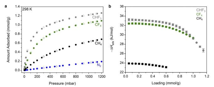
Fig. 3 (a) Adsorption isotherm data for  $CHF_3$ ,  $CF_4$ ,  $CH_4$ , and  $N_2$  in Zn(fba) at 298 K. Filled and open symbols correspond to adsorption and desorption points, respectively. (b) Differential enthalpy of adsorption as a function of loading for  $CHF_3$ ,  $CF_4$ , and  $CH_4$ . Error bars are shown for all data points.
