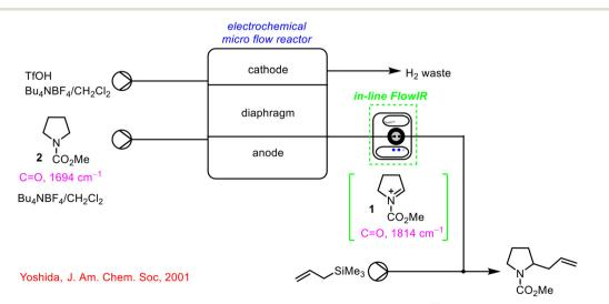
Scheme 1 Early report of the use of FlowIR device in a telescoped continuous process by Yoshida.<sup>33</sup>
