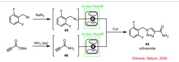
Scheme 16 Continuous flow synthesis of rufinamide using in-line IR reported by Gilmore and co-workers.<sup>56</sup>
