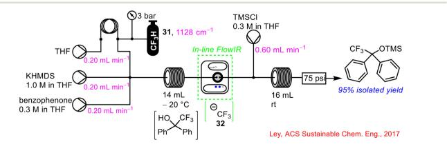
Scheme 12 Reaction monitoring using FlowIR of the use of trifluoromethane 31 to generated functionalised fluorinated compounds in a telescoped flow process.<sup>53</sup>
