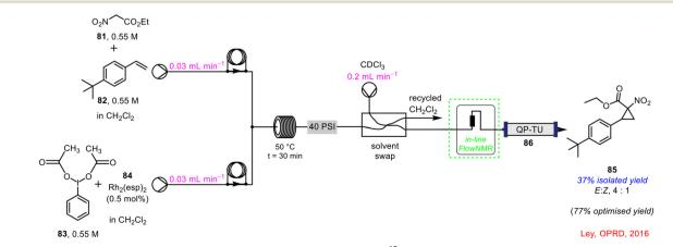
Scheme 31 In-line FlowNMR used in continuous flow cyclopropanation reaction.<sup>15</sup>
