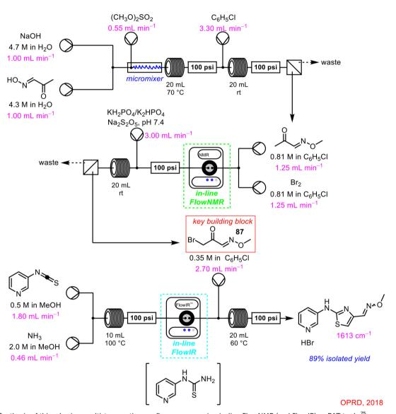
Scheme 33 Synthesis of thiazoles in a multistep continuous flow process using in-line FlowNMR (and FlowIR) as PAT tools.<sup>75</sup>
