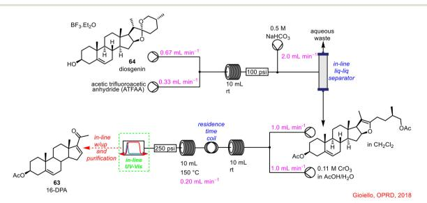
Scheme 23 Telescoped flow synthesis of 16-DPA using in-line UV-vis spectroscopy to monitor reaction completion.<sup>61</sup>
