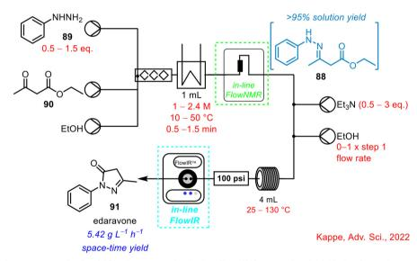
Scheme 35 Telescoped two-step synthesis of API edavarone using in-line FlowNMR to monitor initial imine formation step.<sup>76</sup>
