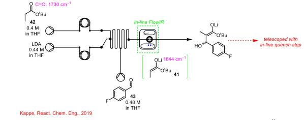
Scheme 15 Simplified schematic of in-line FlowIR cell used by Kappe and co-workers for organolithium transformation.<sup>11</sup>
