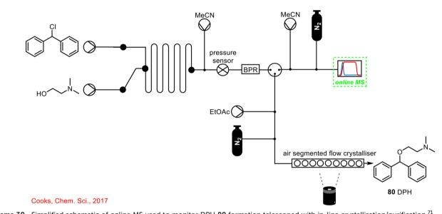
Scheme 30 Simplified schematic of online MS used to monitor DPH 80 formation telescoped with in-line crystallisation/purification.<sup>71</sup>
