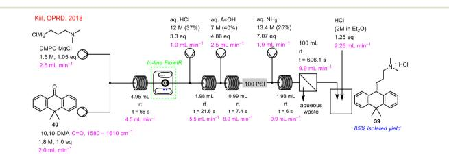
Scheme 14 In-line FlowIR in the telescoped flow synthesis of Melitracen HCl 39 (ref. 9).
