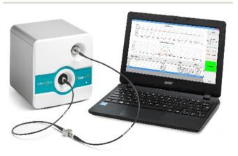
Fig. 3 Image of in-line UV-vis spectrometer by Uniqsis® used in continuous flow (reproduced with permission).
