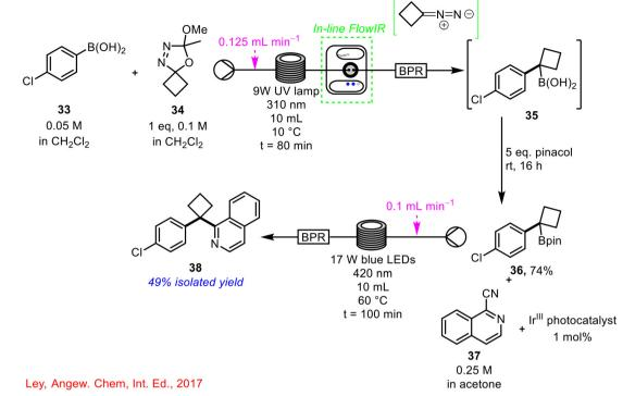
Scheme 13 Synthesis of cyclobutylated isoquinoline compound 38 in a two-step telescoped reaction sequence using in-line FlowIR to monitor the formation of boronic acid 35 (ref. 54).
