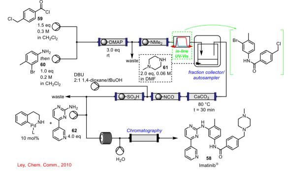
Scheme 22 Telescoped continuous flow synthesis of imatinib 58 incorporating in-line UV-vis spectroscopy to monitor product dispersion following step 1 (amide formation).<sup>60</sup>
