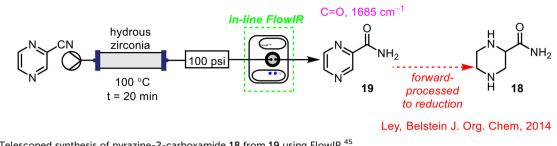
Scheme 6 Telescoped synthesis of pyrazine-2-carboxamide 18 from 19 using FlowIR.<sup>45</sup>
