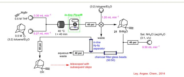
Scheme 7 Initial Grignard step monitored by in-line FlowIR as part of a seven-step telescoped flow sequence.<sup>46</sup>
