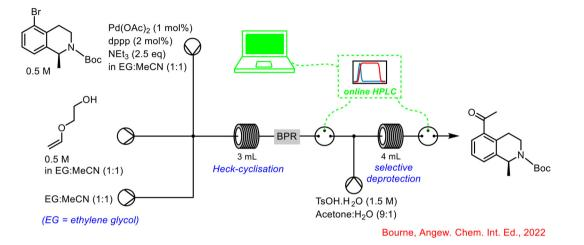
Scheme 27 Integration of online HPLC into self-optimising telescoped reaction by Bourne.<sup>69</sup>
