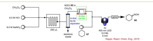
Scheme 24 Telescoped NOCI 65 generation with photochemical synthesis of cyclohexanone oxime 66 using in-line UV-vis spectrometry to monitor NOCI 65 concentration.<sup>64</sup>
