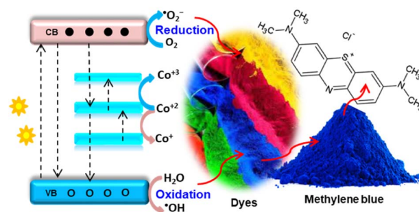
Fig. 3 Scheme showing probable charge transfer within cobalt-doped ZnO: valence to conduction band, cobalt(III) level to host conduction band, cobalt(III) to host valence band, and dopant d–d transition. The charge transfer enhances the electron–hole relaxation time and degrades dye pollutants such as methylene blue by oxidising agents.
