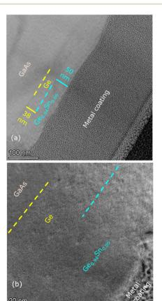
Fig. 5 Cross-sectional TEM micrographs of sample A2: (a) Ge<sub>0.94</sub>Sn<sub>0.06</sub>/ Ge/(100)/2° GaAs heterostructure representing good quality growth of 50 nm  $Ge_{0.94}Sn_{0.06}$  grown over 38 nm thick Ge layer grown on GaAs, where broken lines demarcate similar structure factored Ge and Ge<sub>0.94</sub>Sn<sub>0.06</sub> epilayers, and (b) HR-TEM micrograph affirms the fine quality of the GeSn/Ge heterostructure system.
