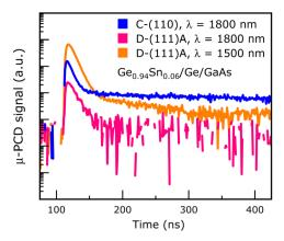
Fig. 10  $\,\mu ext{-PCD}$  measurement data acquired with 1800 nm excitation wavelength for samples C-(110) and D-(111)A. High surface recombination induced noisy signals make the curve inconducive to single exponential fit, with  $R^2$  fitting parameter reaching only 0.41 with 1 as the perfect fit. Similar results are observed at 1500 nm for D-(111)A orientation, indicating its high electrical conductivity, irrespective of excitation wavelength.
