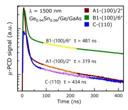
Fig. 8  $\,\mu$ -PCD signal  $\,versus$  time acquired at 300 K with 1500 nm excitation wavelength from samples A1 [(100)/2 $^{\circ}$  Ge $_{0.94}$ Sn $_{0.06}$ ], B1 [(100)/6 $^{\circ}$  Ge $_{0.94}$ Sn $_{0.06}$ ] and C [(110) Ge $_{0.94}$ Sn $_{0.06}$ ]. The corresponding minority carrier lifetimes of  $\sim$ 319 ns,  $\sim$ 481 ns and  $\sim$ 434 ns were obtained by fitting to exponential decay after the initial surface recombination induced decay.
