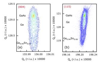
Fig. 4 Reciprocal space maps (RSMs) taken along the (a) (004) and (b) (115) orientations show 100 nm thick  $Ge_{0.94}Sn_{0.06}$  epitaxial layer (sample C) grown on 27 nm Ge layer/(110) GaAs substrate.
