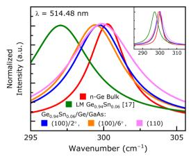
**Fig. 6** Raman spectra recorded from epitaxial  $Ge_{0.94}Sn_{0.06}$  layers of samples A1, B2 and C (compressively strained heterostructures), selectively chosen with different orientations alongside a lattice matched  $Ge_{0.94}Sn_{0.06}$  epilayer.<sup>17</sup> Positive Raman wavenumber shifts (representing compressively strained states) are observed on all three samples A1:  $(100)/2^{\circ}$ , B2:  $(100)/6^{\circ}$ , and C: (110).
