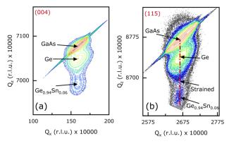
Fig. 3 Reciprocal space maps (RSMs) taken along the (a) (004) and (b) (115) orientations, that shows ~0.81% compressive strain in the 100 nm thick Ge<sub>0.94</sub>Sn<sub>0.06</sub> epitaxial layer (sample B1) grown on 27 nm Ge layer/ (100)/6° GaAs substrate.
