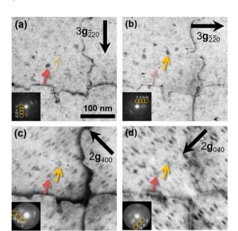
Fig. 6 Invisibility conditions for dislocation loops. (a)  $3g_{220}$  and (b)  $3g_{220}$  images highlight two loops with alternating invisibility. In each, the translucent arrow indicates an invisible loop. In the (c)  $2g_{400}$  and (d)  $2g_{040}$  images, both loops are visible (dark arrows).
