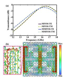
Fig. 6 (a) Comparison of the simulated transmittance for the MFSM and MMFSM under different polarizations. (b) Simulated surface current density of the MMFSM at its resonant frequency under TE polarization. Inset in (b) is the locally amplified surface current density of the red dotted box region.
