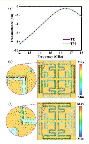
Fig. 3 (a) Simulated transmittance of the MFSM in the Ku band (12-18 GHz) at normal incidence under TE and TM polarization. (b and c) Simulated surface current density of the MFSM at its resonant frequency (16.5 GHz) under (a) TE polarization and (b) TM polarization. Insets in (b) and (c) are the amplified surface current density of the corresponding purple dotted circle regions.
