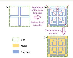
Fig. 2 Schematic of the miniaturization process based on CAFSS: (a) cross-loop aperture, (b) miniaturized cross-loop aperture, and (c) unit cell of MFSMs.
