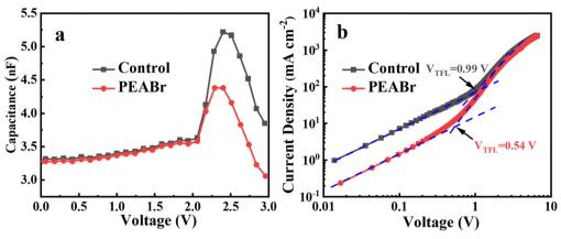
(a) Capacitance-voltage curves of the control and the PEABr-based QLEDs. (b) J-V curves of the EODs with and without PEABr.
