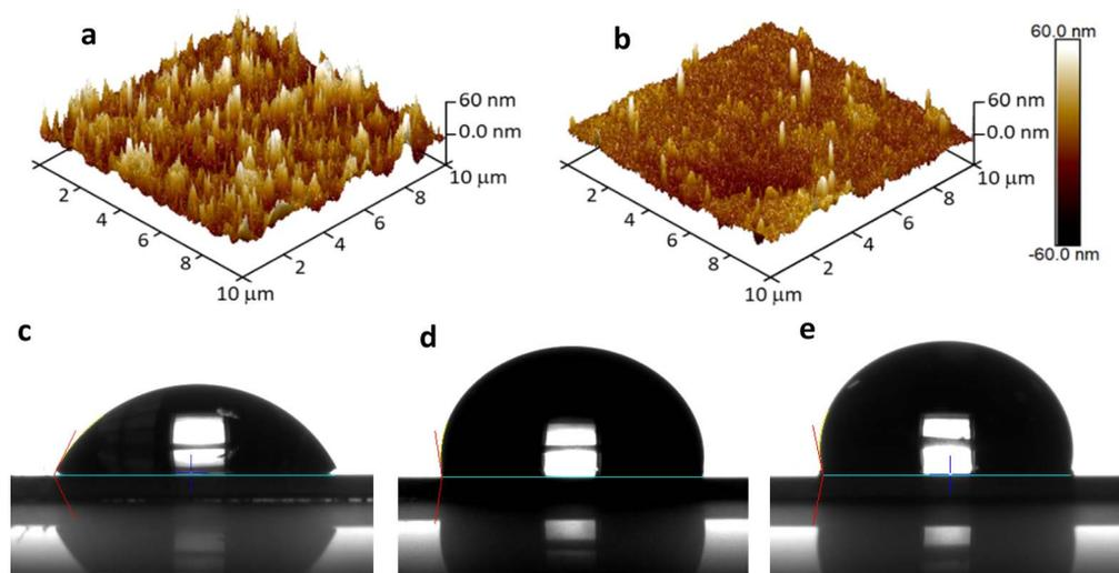
Fig. 8 3D AFM images of QCM-D crystals coated with (a) (Naf/GO-NH<sub>2</sub>)<sub>5</sub> and (b) thermally annealed-(Naf/GO-NH<sub>2</sub>)<sub>5</sub> at 200 °C for 2 h. Contact angles for (c) (Naf/GO-NH<sub>2</sub>)<sub>5</sub>, (d) annealed-(Naf/GO-NH<sub>2</sub>)<sub>5</sub> and (e) Nafion coatings deposited on QCM-D crystals.
