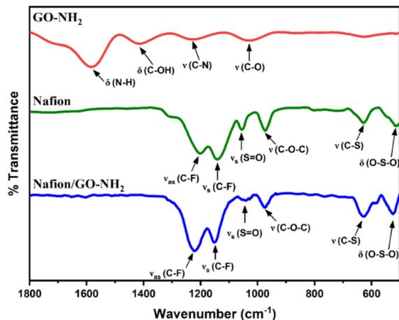
Fig. 2 FTIR spectra of GO-NH<sub>2</sub> (red line), Nafion (green line) and the Nafion/GO-NH<sub>2</sub> nanocomposite (blue line). The pH of the original solutions of GO-NH<sub>2</sub> and Nafion was 2 and 2.7, respectively.
