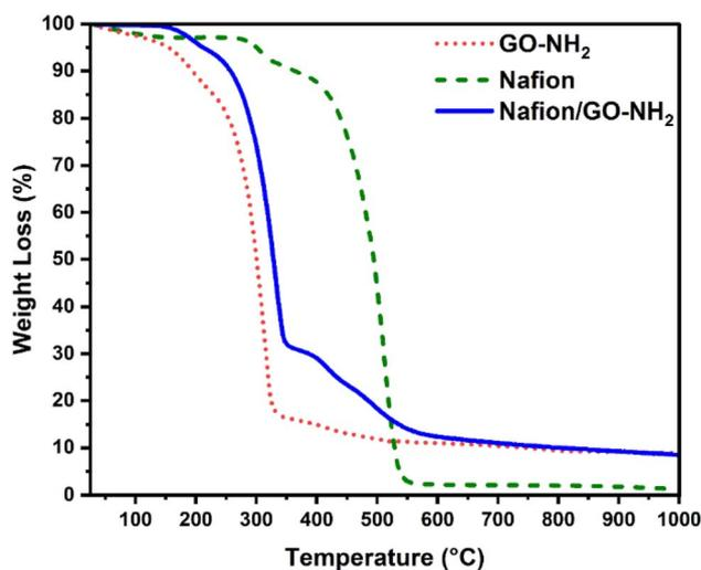
Fig. 5 TGA of GO-NH<sub>2</sub>, Nafion and the Nafion/GO-NH<sub>2</sub> nanocomposite.
