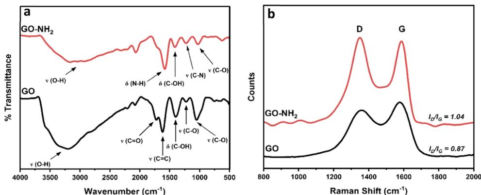
Fig. 1 (a) FTIR and (b) Raman spectra of GO and GO-NH<sub>2</sub>.
