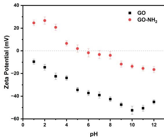
Fig. 3 Zeta potential of 0.005 wt% GO (black squares) and GO-NH<sub>2</sub> (red circles) aqueous dispersions as a function of pH.
