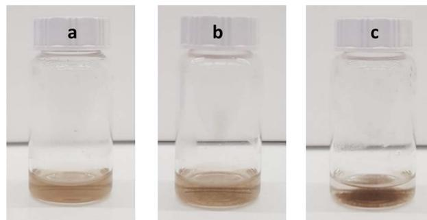
Fig. 4 Optical images of (a) GO-NH<sub>2</sub> and (b) Nafion/GO-NH<sub>2</sub> (1 : 4 ratio) immediately after mixing and (c) Nafion/GO-NH<sub>2</sub> (1 : 4 ratio) 15 min after mixing.
