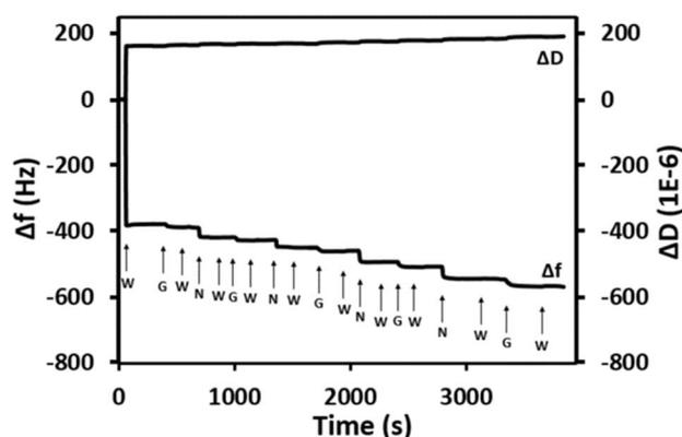
Fig. 6 QCM-D measurements at 25 °C for (Naf/GO-NH<sub>2</sub>)<sub>5</sub> (pH = 2). The letters "W", "G" and "N" indicate the introduction of water, GO-NH<sub>2</sub> and Nafion, respectively.
