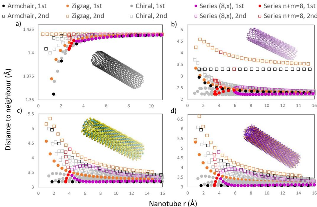
**Fig. 8** Plots of the 1st and 2nd neighbours of the outermost atomic layer for all the chiral and achiral nanotubes in the range  $n, m < 30$  vs. their radius for 4 different materials: (a) SWCNTs, (b) PNTs, (c)  $\text{MoS}_2$  NTs and (d)  $\text{Ti}_3\text{C}_2$  NTs. In the 4 cases, the nanotube series  $(8, m)$  and  $n + m = 8$  were highlighted in red and purple, respectively. The insets show atomistic models to illustrate each NT family.
