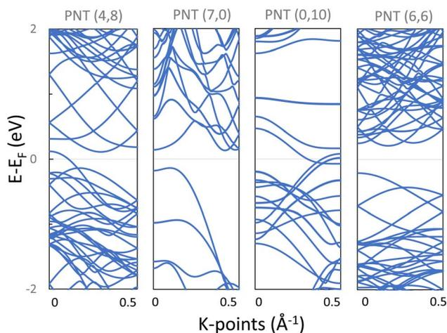
**Fig. 9** Band structure of phosphorene nanotubes, with a metallic character for (4,8) and (0,10), and a semiconductor structure for (7,0) and (6,6), and their bandgaps are 0.27 eV and 0.42 eV, respectively.
