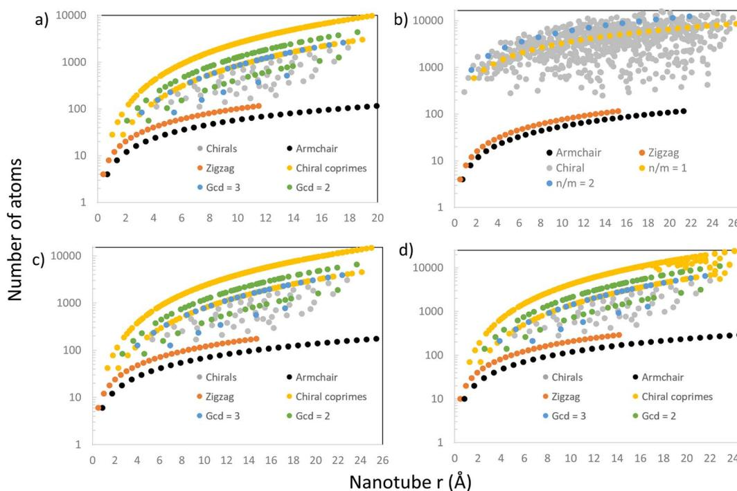
Fig. 6 Plots of the number of atoms for all chiral and achiral nanotubes in the range  $n, m < 30$  vs. their radius for 4 different materials: (a) SWCNTs, (b) PNTs, (c) MoS<sub>2</sub> NTs and (d) Ti<sub>3</sub>C<sub>2</sub> NTs. In a, c, and d, those NTs with  $n, m$  pairs which are coprime are highlighted in yellow, those with g.c.d = 2 in green, and those with g.c.d = 3 in blue. For b, the series of NTs with  $n/m = 1$  and  $n/m = 2$  are highlighted in yellow and blue, respectively.
