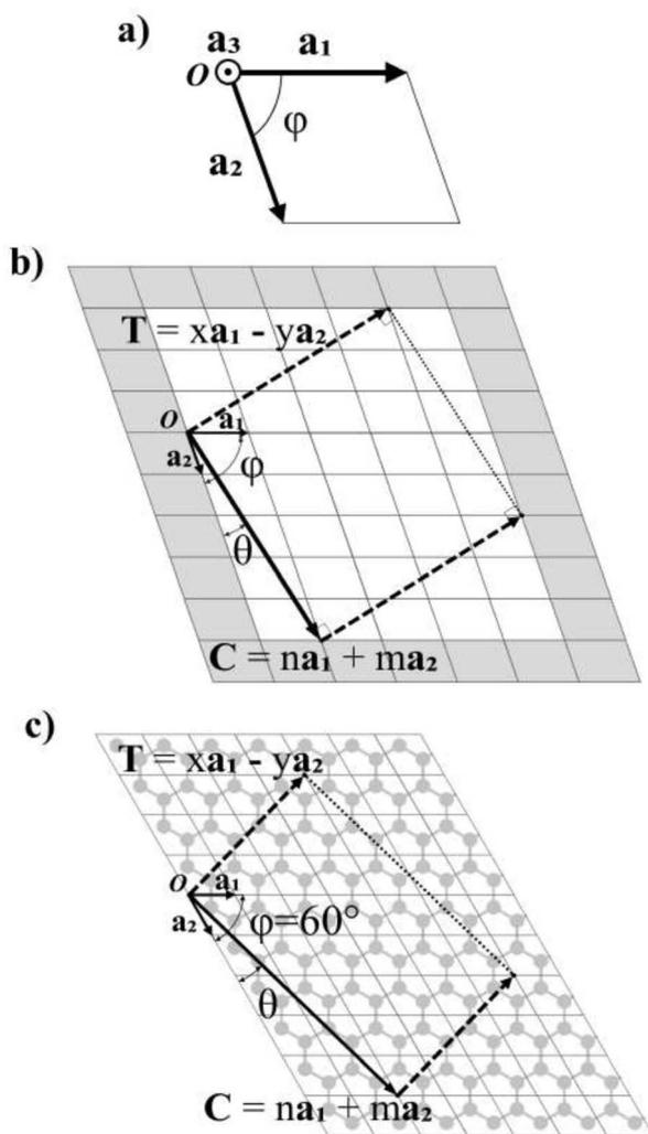
Fig. 1 (a) Unit cell of an arbitrary 2D material.  $\mathbf{a}_1$ ,  $\mathbf{a}_2$  and  $\mathbf{a}_3$  are the vectors of the unit cell.  $\varphi$  is the angle formed between  $\mathbf{a}_1$  and  $\mathbf{a}_2$ . (b) Lattice of a general 2D material with the nanoribbon delimited by the chiral vector  $\mathbf{C}$  and the translational vector  $\mathbf{T}$ . (c) Graphene lattice with a nanoribbon defined by  $\mathbf{C}$  and  $\mathbf{T}$ .
