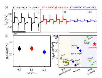
Fig. 4 (a) Pyroelectric response along b-axis under temporal change in temperature of (i) 6.7 °C ( $\Delta T = 1.8$  °C s<sup>-1</sup>), (ii) and 1.6 °C ( $\Delta T = 0.6$  °C s<sup>-1</sup>) (iii) 0.9 °C ( $\Delta T$  = 0.3 °C s<sup>-1</sup>), (b) pyroelectric coefficient as a function of temperature change and (c) comparison of pyroelectric coefficient in different materials (ref. 26-36).
