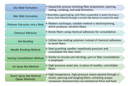
Fig. 4 Nonwoven fabrication processes.
