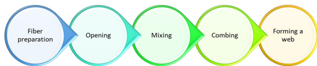
Fig. 3 Steps involved in the formation of nonwovens.
