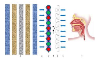
Fig. 11 A scheme of the system. 1 is coupling layers; 2 and 6 show the bidirectional air flows; 3 is electrodes that are used to generate plasma (violet light) filling the space between the layers and the dielectric layer (5); 4 is the switching system that is able to switch on/off the plasma during the expiration/inspiration; 5 is the dielectric material to isolate the body from the electrodes; 7 is mask wearers.<sup>48</sup> Copyright © 2020 American Chemical Society
