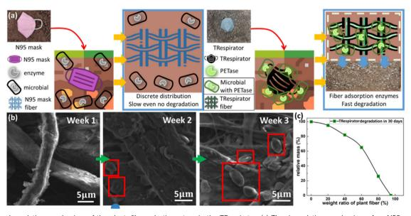
Fig. 14 The degradation mechanism of the plant-fibre-plastic system in the TRespirator. (a) The degradation mechanism of an N95 mask and the TRespirator. (b) SEM images of degrading TRespirator samples from week 1 to week 3. (c) Image about the degradation effect in 30 days with a different weight ratio of plant fibres. 76
