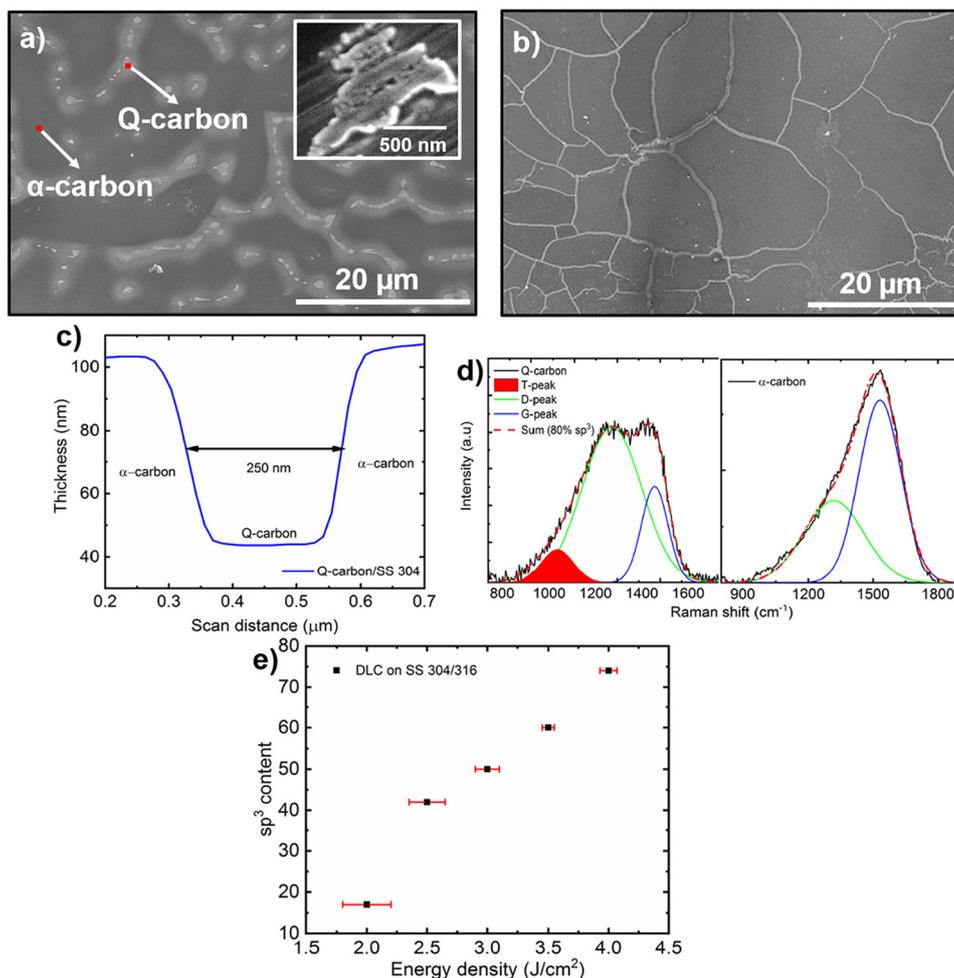
Fig. 9 (a) SEM image demonstrating the formation of Q-carbon on 304 SS, inset shows high-resolution image of Q-carbon in alpha-matrix, (b) SEM image of Q-carbon, (c) surface roughness measurement of Q-carbon, (d) Raman spectra of Q- and alpha-carbon, and (e) correlation between  $sp^3$  content of the DLC as a function of laser energy density used during deposition.<sup>159</sup> Reproduced from ref. 154 with permission from Elsevier, copyright 2020.
