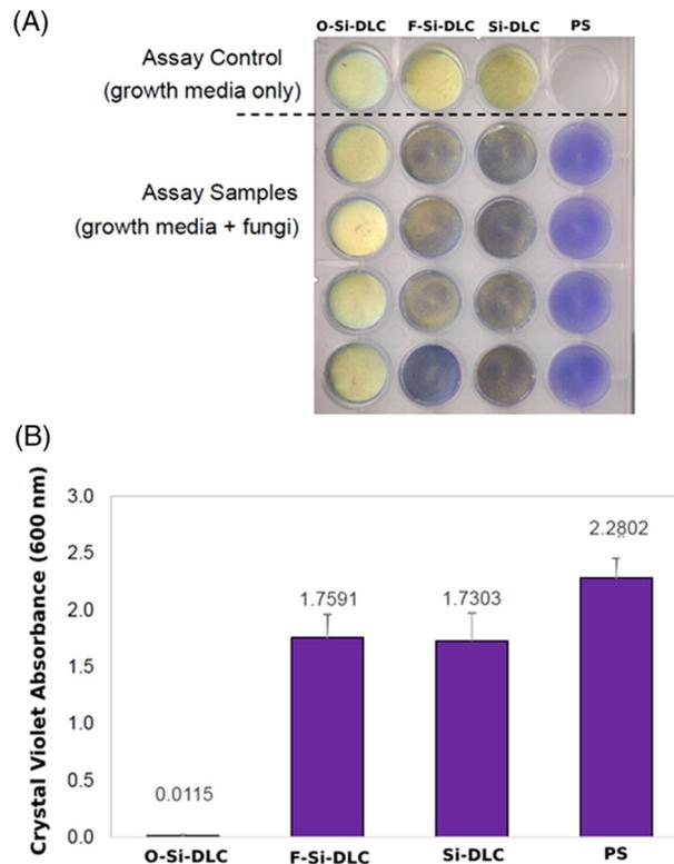
Fig. 8 (A) Images of O-Si-DLC, F-Si-DLC, Si-DLC, and PS with fungal pathogen *Candida albicans* after crystal violet staining. (B) Crystal violet quantification of *C. albicans* on O-Si-DLC, F-Si-DLC, Si-DLC, and PS samples using absorbance measured at 600 nm. (O – oxygen, F – fluorine, PS – polystyrene).<sup>130</sup>
