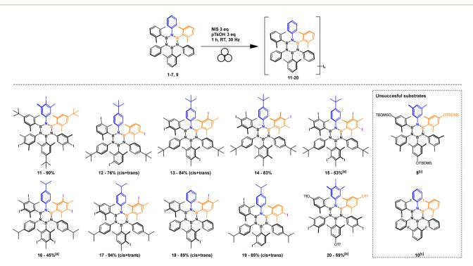
Scheme 2 Substrate scope for the mechanochemical iodination of hexa-aryl borazines. Conditions: borazine 0.08 mmol, NIS 3 eq., TsOH 3 eq., RT, 30 Hz, 1 h. <sup>a</sup> Borazine 0.08 mmol, NIS 3 eq., TsOH 3 eq., RT, 30 Hz, 2 h. <sup>b</sup> Borazine 0.08 mmol, NIS 3 eq., TsOH 3 eq., RT, 30 Hz, 4 h. <sup>c</sup> Formation of an inseparable mixture of unknown products.
