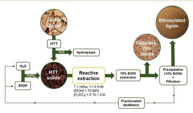
Fig. 1 Schematic representation of reactive extraction (REx)
