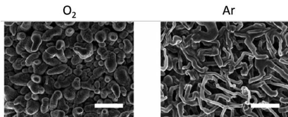
Fig. 5 Effect of O<sub>2</sub> on Li nucleation. SEM images after the first Li plating in Ar (right) and O<sub>2</sub> (left). Scale bar = 10 μm. Reproduced with permission from ref. 4 under the Creative Commons license CC-BY, Copyright 2020.
