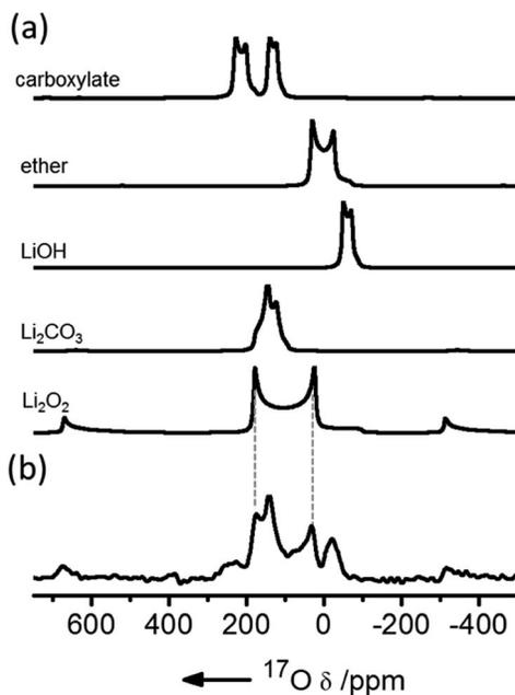
Fig. 2 (a) Simulated  $^{17}\text{O}$  magic angle spinning (MAS) NMR spectra of possible discharge products compared with (b) the experimental spectrum of a cathode extracted from a cell prepared with a 1 M bis(trifluoromethane)sulfonimide lithium (LiTFSI) electrolyte in dimethoxyethane (DME) solution, after discharge, acquired at a field of 21.1 T and fast (60 kHz) MAS. Reproduced with permission from ref. 9 under the Creative Commons license CC-BY, Copyright 2013.
