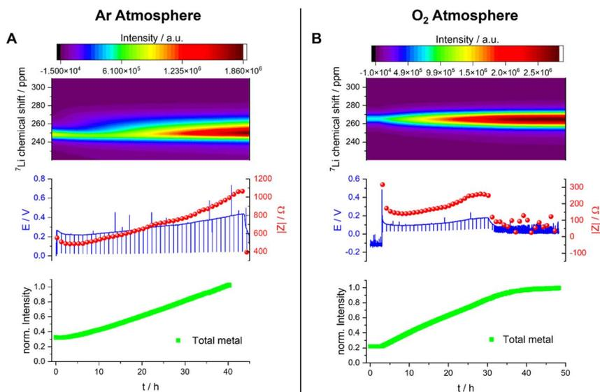
**Fig. 11** Operando NMR spectroscopic measurements of Li-metal plating in symmetrical cells with 1 M LiTFSI in DMSO under Ar (A) and O<sub>2</sub> (B) atmospheres. Operando spectra of the metal between 220 and 310 ppm (top) with the corresponding voltage profile and the impedance magnitude  $|Z|$  at 9 Hz (middle) and normalised intensity of the metal signal (bottom).
