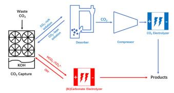
Fig. 1 Schematic representation of the entire CO<sub>2</sub> valorization process of CO<sub>2</sub> electrolyzer and CO<sub>3</sub><sup>2-</sup>/HCO<sub>3</sub><sup>-</sup> electrolyzer.
