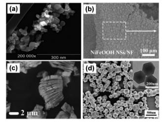
Fig. 3 Morphology of photocatalysts for bioaerosol inactivation. (a) TiO<sub>2</sub> nanoparticles,<sup>56</sup> Reproduced with permission. Copyright 2019, Elsevier. (b) NiFeOOH nanosheets, 75 Reproduced with permission. Copyright 2023, Elsevier. (c) MXene, 63 Reproduced with permission. Copyright 2021, Elsevier. (d) MOF (ZIF-8),85 Reproduced with permission. Copyright 2022, Elsevier.
