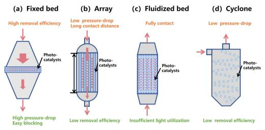
Fig. 9 Assembled photocatalytic reactors of photocatalysts. (a) Fixed bed, (b) array, (c) fluidized bed, and (d) cyclone.
