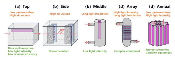
Fig. 10 The assembled light sources in the reactor: (a) top, (b) side, (c) middle, (d) array and (e) annular.
