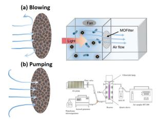
Fig. 13 Performance evaluations of bioaerosol capture. (a) Bioaerosol blowing, 64 reproduced with permission. Copyright 2019, Nature Publishing Group. (b) Bioaerosol pumping,<sup>38</sup> reproduced with permission. Copyright 2022, Elsevier.
