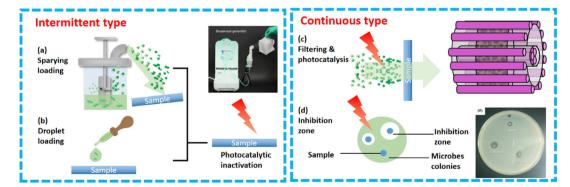
Fig. 14 Performance evaluations of bioaerosol inactivation. (a) Spraying loading with following irradiation.<sup>64</sup> Reproduced with permission. Copyright 2019, Nature Publishing Group. (b) Droplet loading with the following irradiation. (c) Filtering and photocatalysis. (d) Inhibition zone. 127 Reproduced with permission. Copyright 2019, Wiley-VCH GmbH.
