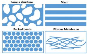
Fig. 8 The structures of photocatalyst carriers.
