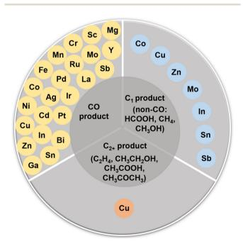
Fig. 2 Schematic diagram of the reported elements in SACs for CO<sub>2</sub>RR.
