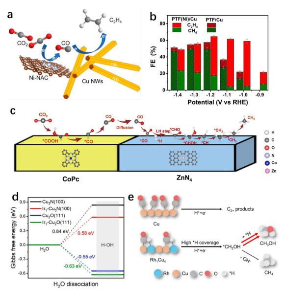
Fig. 8 (a) Schematic diagrams of the tandem systems of Cu/Ni-NAC hybrid catalysts.  $^{154}$  (b) Faradaic efficiency of  $C_2H_4$  and  $CH_4$  at different potentials on PTF(Ni)/Cu and PTF/Cu. 155 (c) A proposed reaction mechanism for the production of CH<sub>4</sub> over CoPc@Zn-N-C. 158 (d) Calculated  $\Delta G$  for the H<sub>2</sub>O dissociation process. 162 (e) Mechanism of CH<sub>3</sub>OH formation on the Rh<sub>1</sub>Cu<sub>4</sub> catalyst. 161
