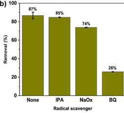
Fig. 6 (a) Percentage of TET removal upon C600KT recycling and (b) effect of radical scavengers on TET removal from aqueous solution with C600KT after 60 min. Fig. 6a does not have error bars because each bar represents a single experiment. The error bars in Fig. 6b are small showing a high reproducibility.
