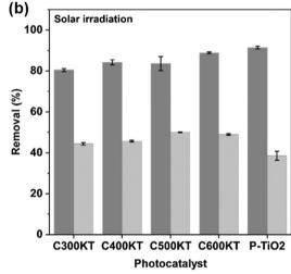
Fig. 7 Mineralization and degradation of TET in aqueous solution by P-TiO<sub>2</sub> and all composites under (a) UVB and (b) solar irradiation for 120 min. Dark grey is degradation, light grey indicates mineralization in both panels.
