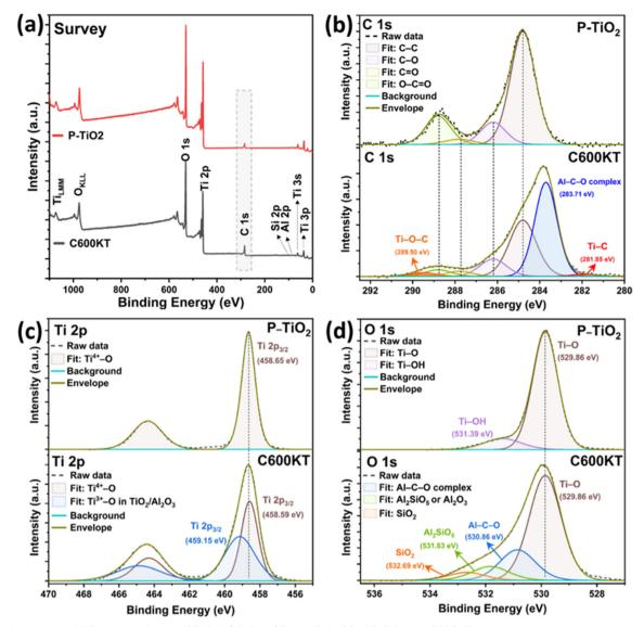
Fig. 3 High-resolution XPS spectra of survey (a), C 1s (b), O 1s (c), and Ti 2p (d) of P-TiO2 and C600KT, respectively.
