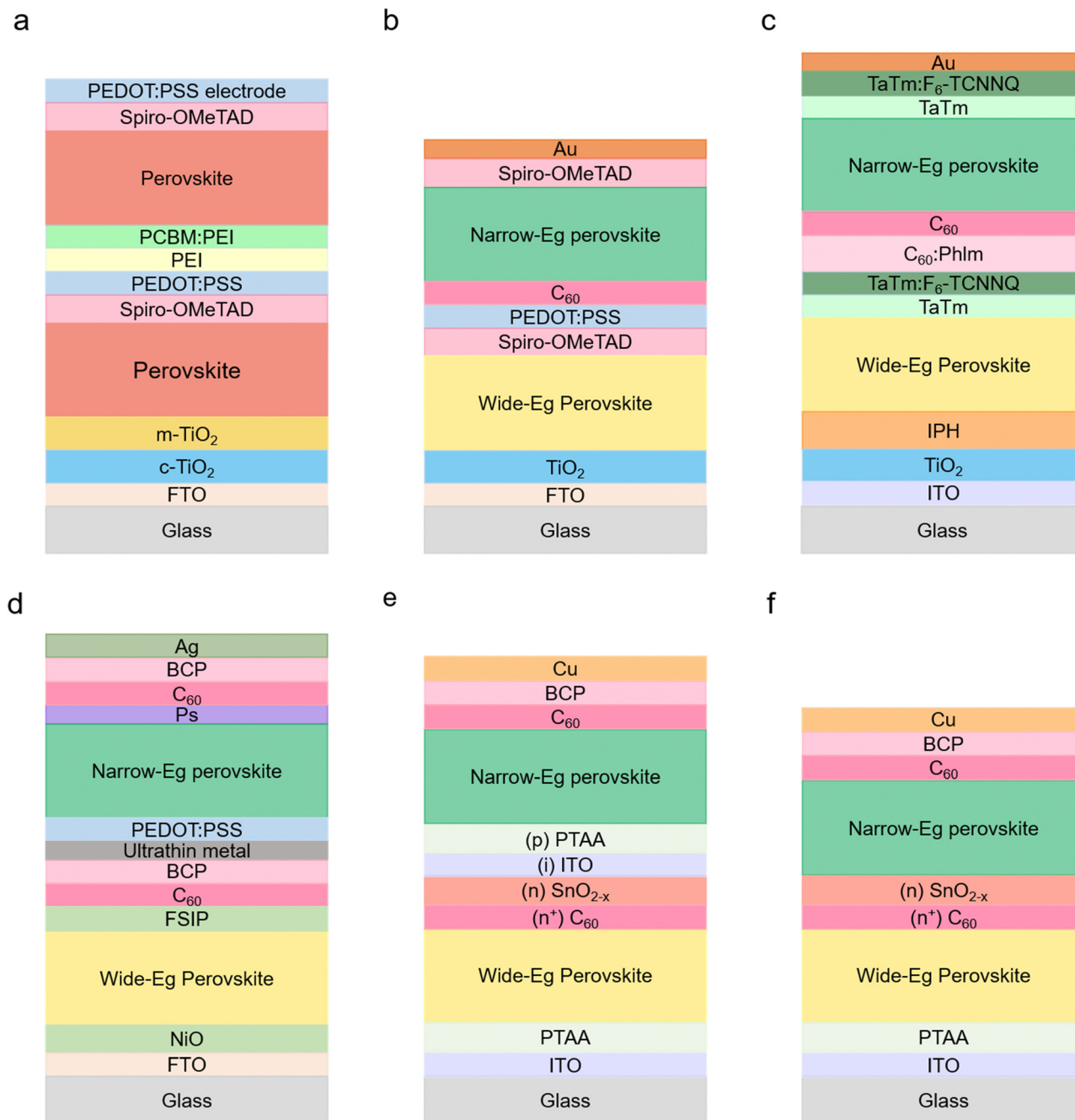
Fig. 9 Several configurations of charge recombination layers. (a) Device configuration including the charge recombination layer of spiro-MeOTAD/PEDOT:PSS/PEI (polyethylenimine)/PCBM:PEI. © 2020. Royal Society of Chemistry. All rights reserved. 174 (b) Cell structure including the charge recombination layer of Spiro-MeOTAD/PEDOT:PSS/C 60 . © 2017. American Chemical Society All rights reserved. 175 (c) Device structure including an organic dopant (F 6 -TCNNQ) in TaTm for the charge recombination layer configuration. © 2016. John Wiley and Sons. All rights reserved. 176 (d) Device configuration including the charge recombination layer of (fluoride silane and polyethylenimine ethoxylated (PEIE) in trichloro(3,3,3-trifluoropropyl)silane) FPTS/C 60 /BCP/Cu:Au alloy/PEDOT:PSS. © 2018. John Wiley and Sons. All rights reserved. 177 (e) Device structure before simplifying the charge recombination layer of C 60 /SnO 2-x /ITO/PTAA. (f) Device structure after simplifying the charge recombination layer of C 60 /SnO 2-x . © 2020. Springer Nature. All rights reserved. 178
