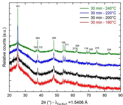
**Fig. 1** pXRD patterns of anatase TiO<sub>2</sub> after synthesis at 180 (red), 200 (black), 220 (blue) and 240 °C (green).
