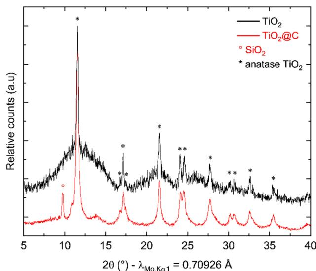
**Fig. 3** pXRD patterns before (black) and after (red) heat treatment under H<sub>2</sub>.
