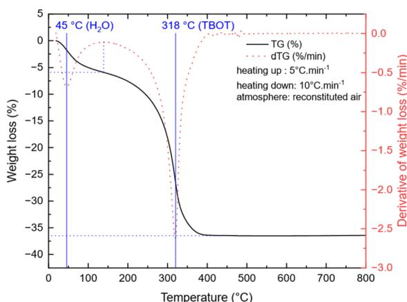
**Fig. 2** TGA of TNPs after synthesis (180 °C, 30 min).
