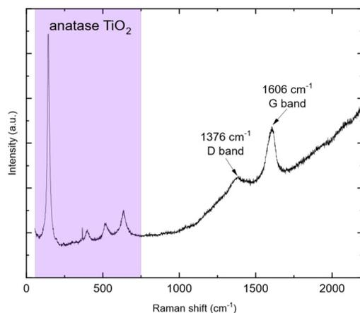
Fig. 5 Raman spectrum of  $\text{TiO}_2\text{@C}$  (457 nm wavelength).
