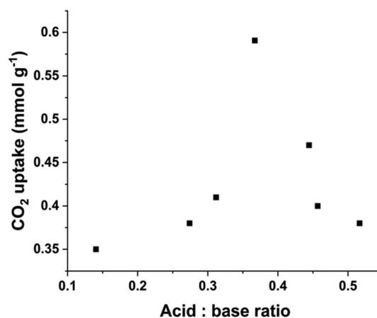
Fig. 5 CO<sub>2</sub> capture as a function of acid:base ratio of LDOs calcined at 400 °C.
