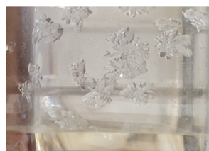
Fig. 2 A collection of N 2 O 5 crystal clusters. Note that the clusters are usually up to 1–1.5 cm across.
