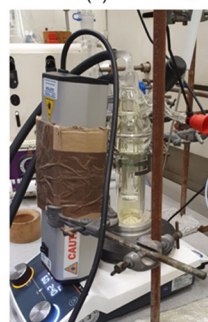
Fig. 6 The apparatus with the UV modification to the Deville method. Note that the colour has no NO 2 character and that the N 2 O 5 condensers immediately after it has been produced. The UV lamp (left side) has been partially blocked to only irradiate the lower part of the sublimator with the silver nitrate.
