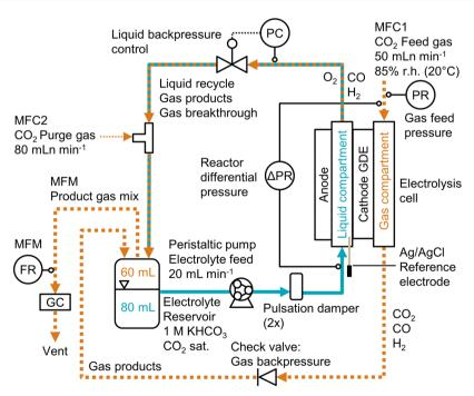
Fig. 1 Process flow diagram for  $CO_2$  electrolysis setup. The backpressure of the electrolyte stream was controlled (PC) before it was mixed with the purge gas and recirculated. The differential pressure,  $\Delta p$ , across the GDE was measured between the catholyte and gas compartment ( $\Delta$ PR). The Faradaic efficiency was determined by recording the product gas flow rate (FR) with a mass flow meter (MFM) and analyzing the gas composition by gas chromatography (GC).
