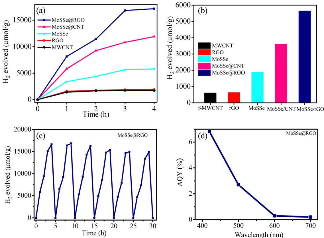
Fig. 6 (a) Photocatalytic H<sub>2</sub> evolution data of the bare MWCNTs, RGO, MoSe<sub>2</sub>, MoSe<sub>2</sub>@CNT, and MoSe<sub>2</sub>@RGO nanocomposites; (b) bar diagram showing the comparison of the HER activities of the samples; (c) cycling stability curve for MoSe<sub>2</sub>@RGO nanocomposites and (d) AQY measured on the optimum MoSe<sub>2</sub>/RGO catalyst at 420, 500, 600 and 700 nm.
