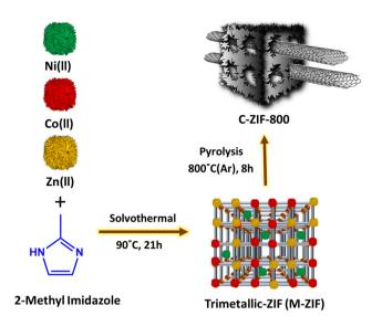
Scheme 1 Illustration of the solvothermal treatment of M-ZIF followed by pyrolysis at 800 °C under argon.
