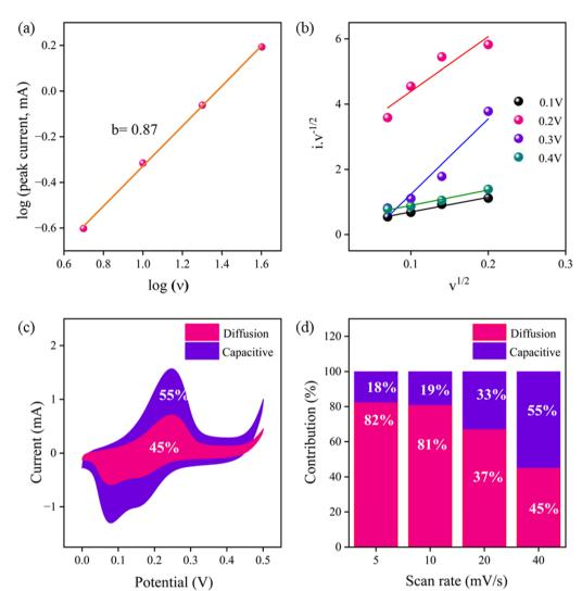
Fig. 4 (a)  $\log(v)$  vs.  $\log(\text{peak current})$  profile for finding the *b*-value. (b)  $i/v^{1/2}$  vs.  $v^{1/2}$  profile. (c) Percentage contribution of surface capacitance and diffusion-controlled capacitance for C-ZIF-800 in 1 M KOH electrolyte at 40 mV s<sup>-1</sup>. (d) Bar diagram representing percentage contributions at various scan rates.
