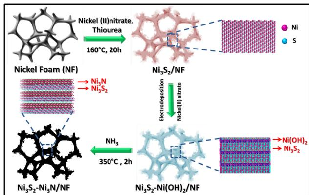
Scheme 1 The synthesis strategy of the Ni<sub>3</sub>S<sub>2</sub>-Ni<sub>3</sub>N/NF catalyst.
