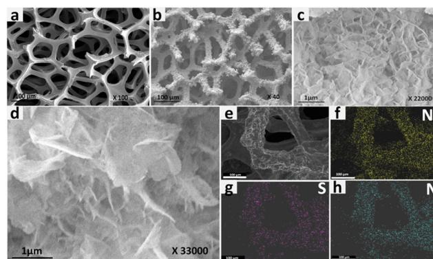
Fig. 2 The SEM images of (a) bare nickel foam and (b)  $\text{Ni}_3\text{S}_2\text{-Ni}_3\text{N}$  heterostructure nanosheets over NF; (c and d) the sheet-like morphology of  $\text{Ni}_3\text{S}_2\text{-Ni}_3\text{N}$  and (e-h) elemental mapping of  $\text{Ni}_3\text{S}_2\text{-Ni}_3\text{N}$  showing the presence of all the elements uniformly over the catalyst surface.
