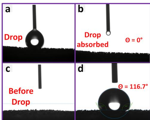
Fig. 4 (a and b) The contact angle measurement of  $\text{Ni}_3\text{S}_2$ - $\text{Ni}_3\text{N}$  showing superhydrophilic behavior with a contact angle of  $0^\circ$ . (c and d) Bare nickel foam (NF) showing hydrophobic behavior with a contact angle of  $116.7^\circ$ .
