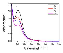
Fig. 5 UV-vis spectra of Au<sup>3+</sup> solution at different time during the swelling of (A) PNIPAM (B) PAAM. 0 h (black line), 3 h (red line), 5 h (blue line), and 30 h (pink line).
