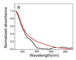
Fig. 1 UV-vis spectra of: (A) Au nanomaterials obtained in PNIPAM (Au-PNIPAM NCs, black line) and PAAM (Au-PAAM NCs, red line) hydrogels. (B) NIPAM (black line) and PAAM (red line) hydrogels.
