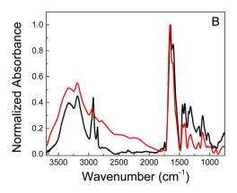
Fig. 3 FT-IR spectra of (A) pure PNIPAM (black) and Au-PNIPAM NCs (red) lyophilizated materials. (B) Pure PAAM (black) and Au-PAAM NCs (red) lyophilizated materials
