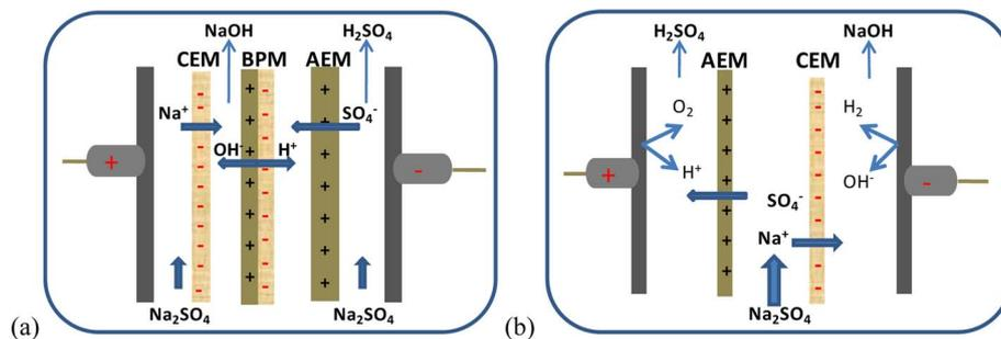
Fig. 7 Schematic representations of bipolar membrane electrodesalination (a) and electro-electrodesalination (b).
