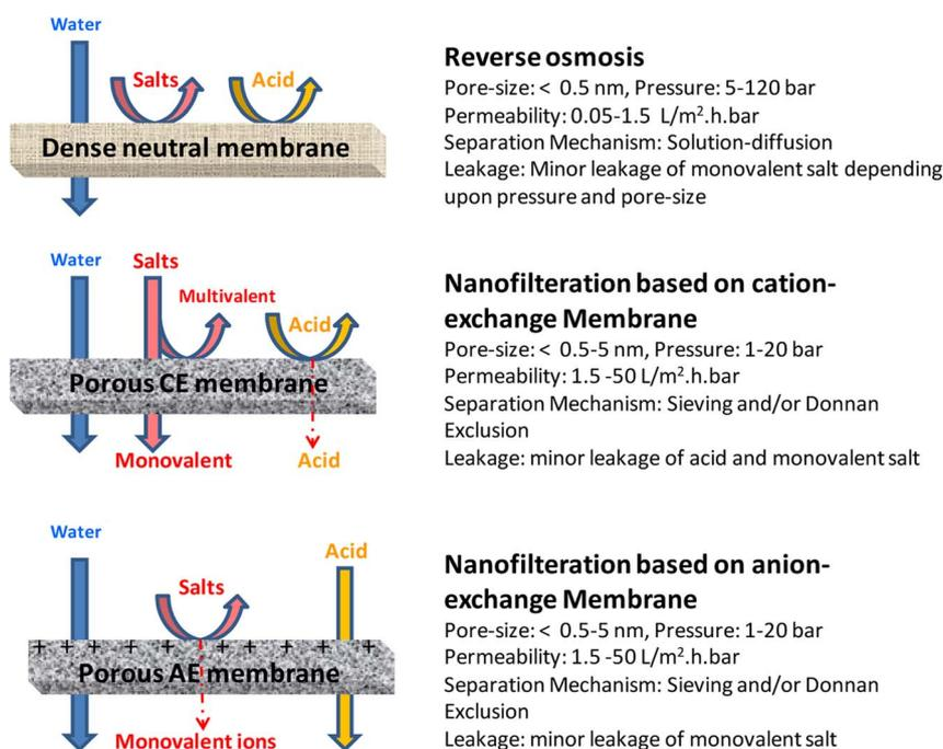
Fig. 4 Schematic illustration of separation of acid, salts, water in aqueous waste using reverse osmosis (RO) and nanofiltration (NF) membrane-based processes.
