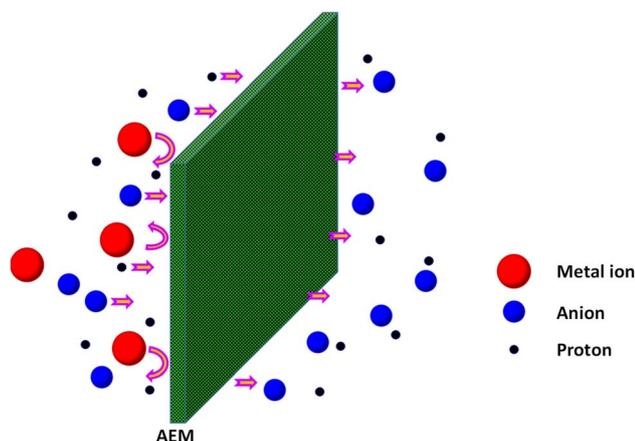
Fig. 5 Basic principle of a diffusion dialysis process.
