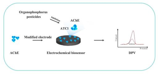
Fig. 2 The principle of the enzyme sensor.
