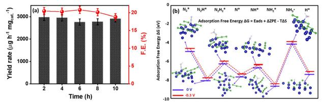
Fig. 4 (a) F.E. and NH<sub>3</sub> yield obtained after chronoamperometry tests performed for 10 h under N<sub>2</sub>-saturated 0.1 M KOH for Co<sub>2</sub>B (1:8). (b) Free energy diagrams of the NRR distal pathway on  $Co_2B$  surface (Co active site) at applied potentials of 0 and -0.3 V and H<sup>+</sup> adsorption at identical potentials
