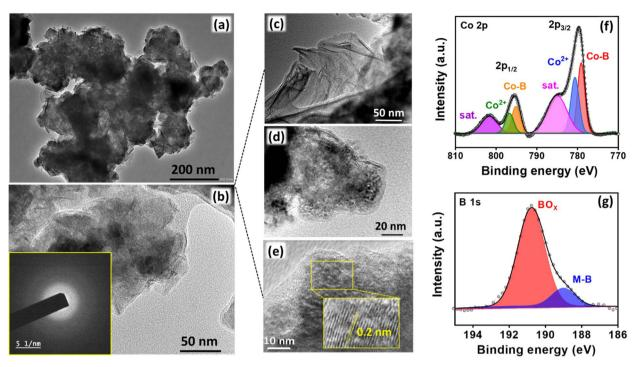
Fig. 3 (a–e) HR-TEM images of  $Co_2B$  (1:8) at different magnifications (inset of (b) shows SAED pattern for  $Co_2B$  (1:8) revealing an amorphous nature and inset of (e) shows d-spacing corresponding to  $Co_2B$  with short range atomic arrangement at few locations). (f) Deconvoluted XP spectra of Co 2p and (g) XP spectra of B 1s for  $Co_2B$  (1:8) catalyst.
