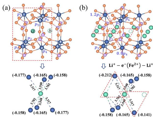
Fig. 3 Partial charges of an electron for (a) the isolated state and (b) the aggregated state of  $\text{Li}^+$  in the  $\text{LiFePO}_4$  structure. The dimension unit of  $\text{Li}^+e^-$  ( $\text{Fe}^{2+}$ ) distance is  $\text{\AA}$ .
