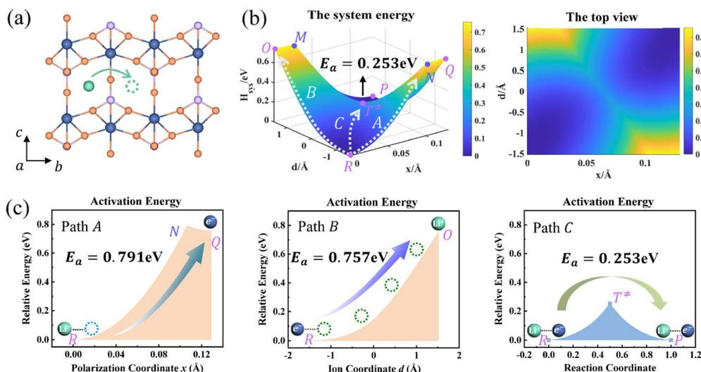
Fig. 4 (a) Structure diagram of Li<sup>+</sup> hopping along the *b*-axis in FePO<sub>4</sub>. (b) Potential energy surface based on the Hamiltonian model (left) and its top view (right) for ion hopping and electron transfer. (c) Potential energy curves of paths A, B, and C.
