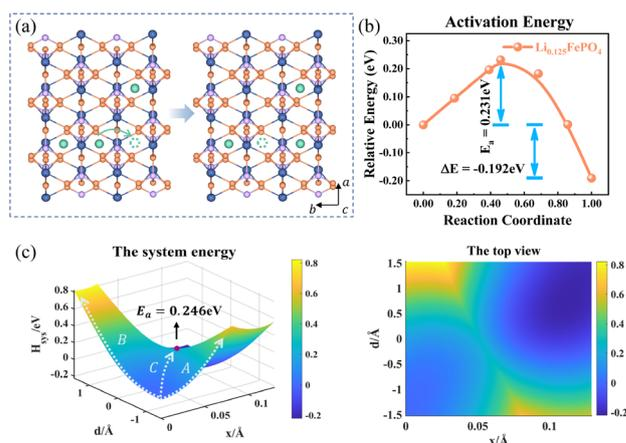
Fig. 5 (a) Structure diagram of the initial and final states of Li<sup>+</sup> hopping. (b) The activation energy calculated using the NEB for asymmetric ion hopping in Li<sub>0.125</sub>FePO<sub>4</sub>, and (c) potential energy surface based on the Hamiltonian model (left) and its top view (right) for ion transport and electron transfer.
