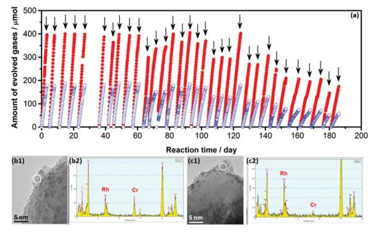
Fig. 4 (a) Long-term measurement of  $Rh_{2-\nu}Cr_{\nu}O_3/GaN:ZnO$  photocatalyst for overall water splitting under visible light. (b and c) Combination of TEM and EDS analysis for the  $Rh_{2-\nu}Cr_{\nu}O_3/GaN$  photocatalyst (b) before and (c) after deactivation. Reproduced from ref. 51, copyright 2012, American Chemical Society.
