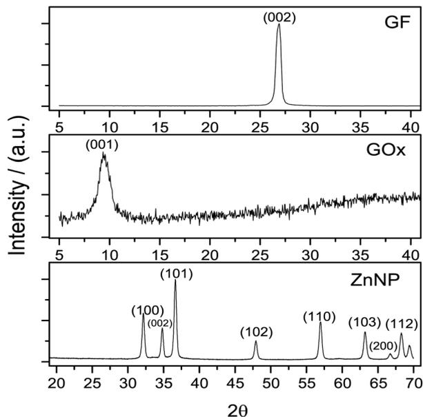
Fig. 1 Normalized XRD diffraction patterns from graphite (GF), graphene oxide (GOx) and zinc nanoparticles (ZnNP). Graphite has a characteristic peak at  $2\theta = 26^\circ$  whilst the GOx presents its peak at  $2\theta = 10^\circ$ . XRD pattern from ZnNP exhibited characteristic peaks at the angles  $2\theta = 31, 34, 36, 47, 56, 62, 66, 68$  and  $69^\circ$ .
