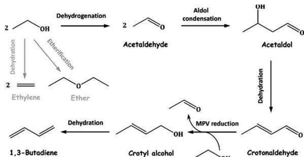
Fig. 8 Dehydration and condensation reaction route of ethanol.
