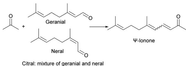
Fig. 20 Condensation reaction of acetone with germanial.
