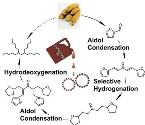
Fig. 10 Condensation reaction of furfural and acetone.
