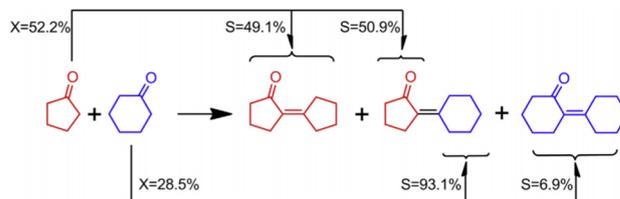
Fig. 22 Condensation reaction of cyclopentanone and cyclohexanone.
