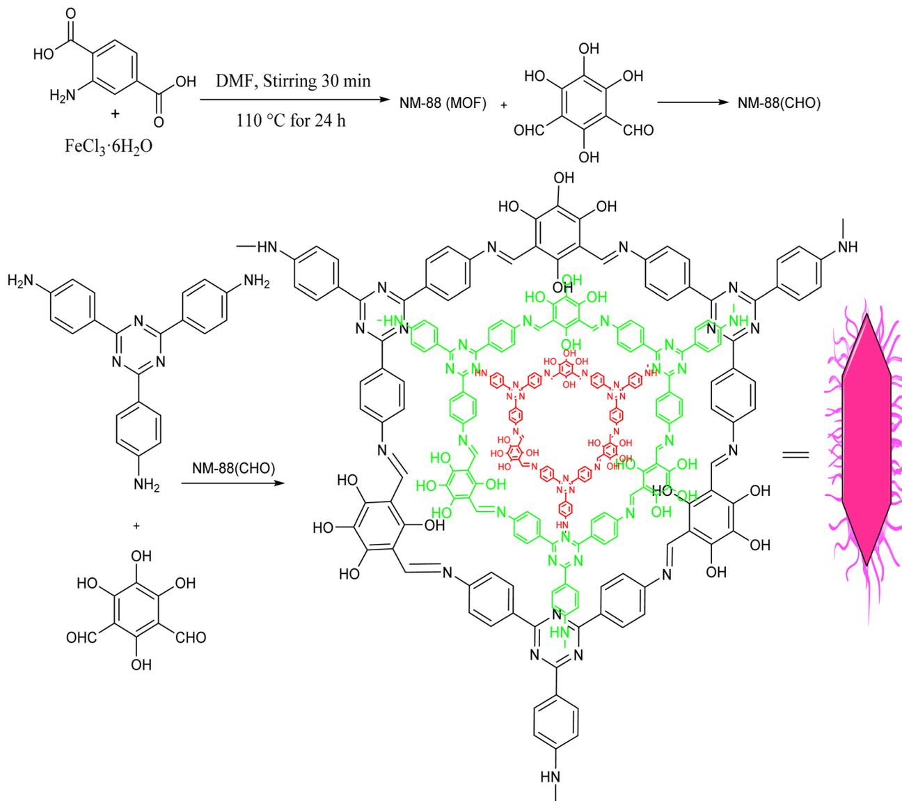
Fig. 9 The preparation of NMC<sub>TP-TTA</sub> hybrid nanozyme. Reproduced with permission from ref. 22.
