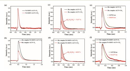
Fig. 4 The in situ TPV patterns of different materials in N<sub>2</sub>-saturated ACN solution (black curve) and CO<sub>2</sub>-saturated ACN solution (red curve). (a) Ni-MOF1. (b) Ru complex/Ni-MOF1 (black curve) and Ru complex (red curve) in N2-saturated ACN solution. (c) Ru complex. (d) Ru complex/Ni-MOF1. Charge annihilation process of (e) the Ru complex and (f) Ru complex/Ni-MOF1.
