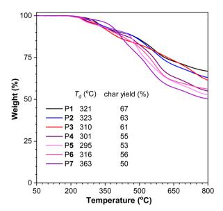
Fig. 3 TGA curves of polythioamides P1-P7 with a heating rate of 10 °C min<sup>-1</sup> under nitrogen.
