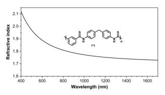
Fig. 5 The wavelength dependence of the refractive index of the thin film of P1.
