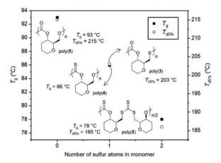
Fig. 5 Glass transition and degradation temperatures of poly(2–5) vs. the quantity of sulfur atoms in their monomers. Notable omissions include: poly(3) (no  $T_a$  detected) and poly(4) ( $T_{d5\%}$  = 136 °C).
