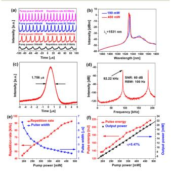
**Fig. 6** Q-switched experimental results: (a) digital oscilloscope image; (b) optical spectrum; (c) single-pulse shape; (d) the RF spectrum; (e) the change of pulse duration and repetition rate; and (f) the variation output power and single-pulse energy.
