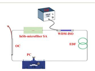
Fig. 5 The setup of the Q-switched EDF laser.
