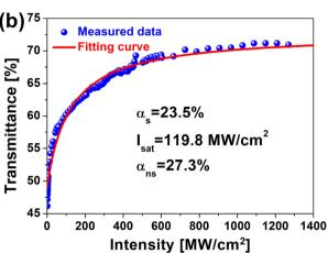
Fig. 4 (a) The balanced twin-detector measurement and (b) the non-linear optical transmittance properties of the InSb-microfiber SA.
