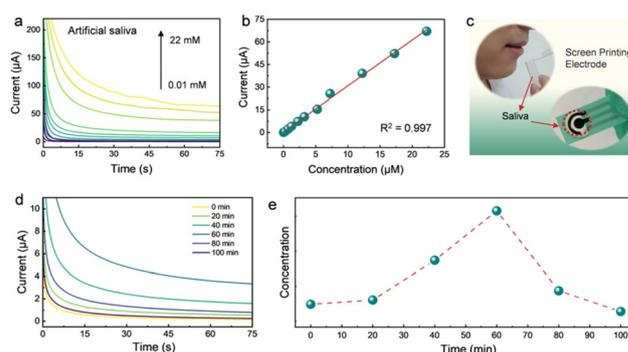
**Fig. 4** Analysis of AA in personalized saliva. (a) Responses of the Rh SAzyme sensor to different concentrations of AA in artificial saliva, and (b) the corresponding concentration–current fitted curve. (c) Schematic diagram of the analysis of saliva samples with the Rh SAzyme sensor. (d) Response of a Rh SAzyme sensor to AA in saliva before and after taking 1 g AA pills at 20 min intervals. (e) The corresponding signal response vs. time.
