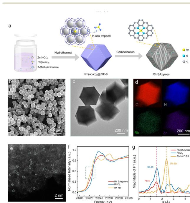
**Fig. 1** The design and characterization of Rh SAzymes. (a) Schematic illustration of the preparation process. (b) SEM image, (c) TEM image, (d) EDS element maps, and (e) aberration-corrected HAADF-STEM image of the Rh SAzymes. (f) XANES and (g) EXAFS spectra of the Rh SAzymes, RhCl<sub>3</sub>, and Rh foil at the Rh k-edge.
