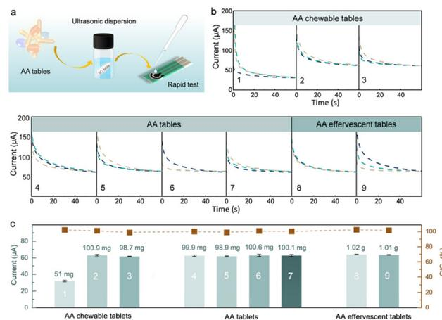
**Fig. 5** Analysis of AA in nutritional products. (a) Illustration of the Rh SAzyme sensor for onsite detection of AA in nutritional products. (b) Response of the Rh SAzyme sensor to various types of AA products. (c) Test results and comparison with theoretical values.
