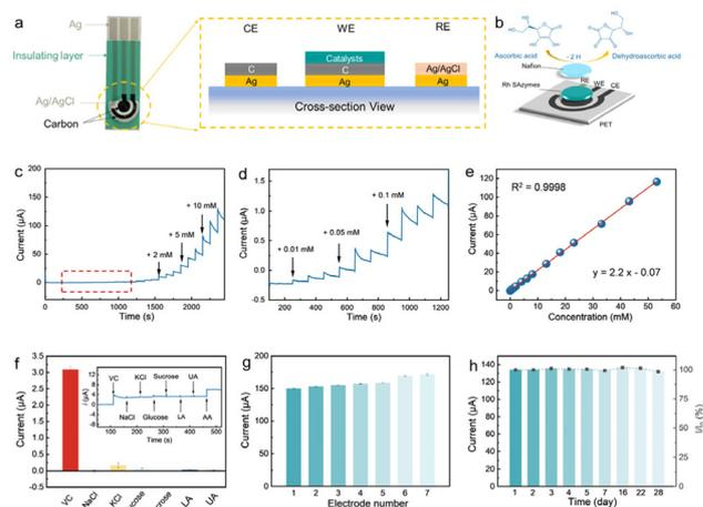
**Fig. 3** Miniaturized electrochemical sensor. (a) The optical image and cross-section view of a screen-printed sensor. (b) Scheme of the modified working electrode. (c) Amperometric responses of the Rh SAzyme sensor to the successive addition of AA, and (d) a zoomed-in area of the red square region. (e) The corresponding concentration–current fitted curve. (f) The selectivity, (g) reproducibility and (h) stability tests of the Rh SAzyme sensor.
