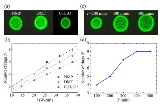
Fig. 2 (a) Complete ring patterns with VP Ns dispersed in three different solvents at  $I = 31.7 \text{ W cm}^{-2}$ . (b) Intensity dependence of the number of rings for VP Ns dispersed in three different solvents. (c) Complete ring patterns for VP Ns dispersed in NMP at I = 37.5 W cm<sup>-2</sup> with three ultrasonic times T. (d) T-Dependence of the number of rings for VP Ns dispersed in NMP at I = 37.5 W cm<sup>-2</sup>.
