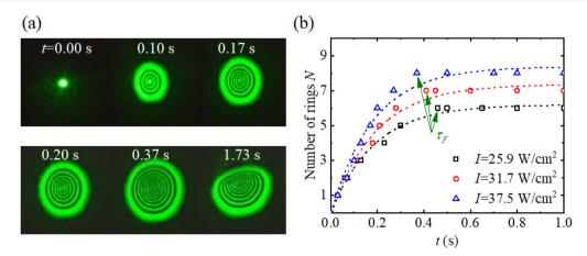
Fig. 3 (a) The self-diffraction ring patterns of VP nanosheet dispersion in NMP recorded at different times t with I = 37.5 W cm<sup>-2</sup>. (b) The evolution of the number of rings N over time t at three different intensities.
