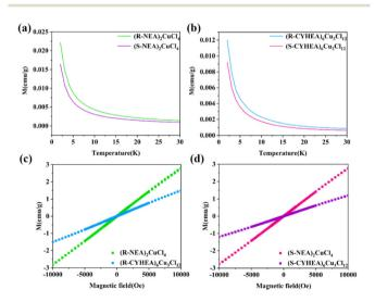
Fig. 2 Temperature-dependent magnetization of (a) (R-/S-NEA)<sub>2</sub>CuCl<sub>4</sub> and (b) (R-/S-CYHEA)<sub>6</sub>Cu<sub>3</sub>Cl<sub>12</sub>. Magnetic field-dependent magnetization of (c) R-type and (d) S-type perovskites.
