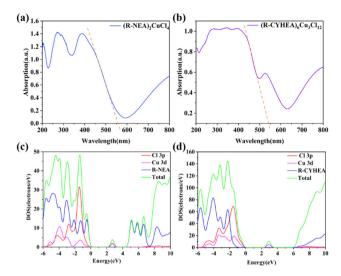
Fig. 4 The UV-Vis spectrum of (a) (R-NEA)<sub>2</sub>CuCl<sub>4</sub> and (R-CYHEA)<sub>6</sub>Cu<sub>3</sub>Cl<sub>12</sub> single crystals. The DOS of (c) (R-NEA)<sub>2</sub>CuCl<sub>4</sub> and (d) (R-CYHEA)6Cu3Cl12.
