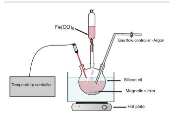
Fig. 1 Experimental setup of the thermal decomposition process.
