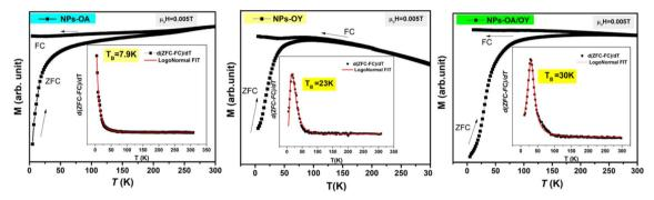
Fig. 5 ZFC/FC magnetization curves and the blocking temperature  $T_{\rm B}$ .
