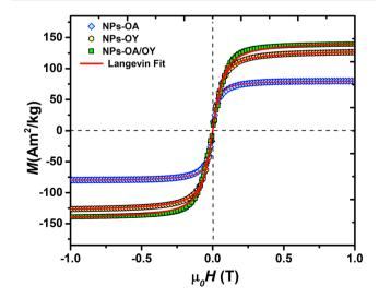
Fig. 3 Room temperature magnetization of the Fe-based NPs with different surfactants.
