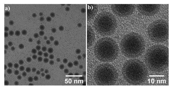
Fig. 8 (a) Low and (b) high magnification bright field TEM images of the nanoparticles after surface functionalization.
