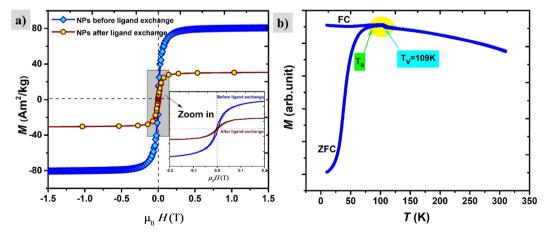
Fig. 10 (a) Magnetization curves of nanoparticles before and after ligand exchange, zoom in (the inset). (b) The ZFZ/FC curve of nanoparticles after ligand exchange, showing the blocking temperature  $T_{\rm B}$  and  $T_{\rm V}$  Verwey transition.
