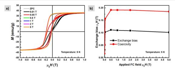
Fig. 11 M(H) loops (a) measured at 5 K temperature after field cooling in different applied magnetic fields up to  $\mu_0 H = 5$  T. (b) Exchange bias field and coercivity as a function of the applied magnetic field during cooling.
