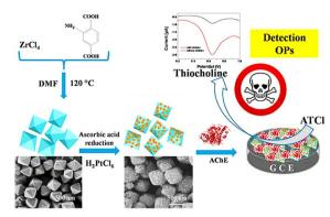
Fig. 15 Schematic representation of detection of organophosphates using Pt@UiO-66-NH<sub>2</sub>@GCE (reproduced with permission from Li Ma et al.<sup>97</sup> Copyright 2019 Elsevier).
