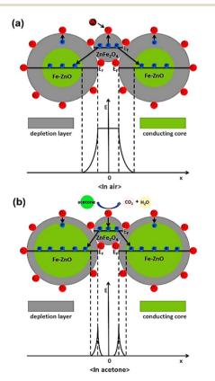
Fig. 14 Schematic diagram of the structure and band for the ZnFe<sub>2</sub>O<sub>4</sub>/ Fe-ZnO nanocomposite-based sensor (a) in air and (b) in acetone (reproduced with permission from ref. 90. Copyright 2020 Elsevier).
