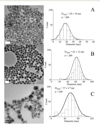
Fig. 3 TEM images and histograms for  $D_{\text{TEM}}$  of NFs prepared from [Mn(acac)<sub>3</sub>]/[Fe(acac)<sub>3</sub>] = (A) and (B) 1 & 3, respectively at 200 °C, (C) ratio = 7 at 250 °C.
