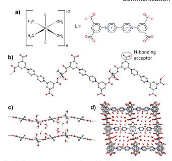
Fig. 1 Crystal structure of Ni-ZW-MOF. a) Octahedral coordination environment of Ni<sup>2+</sup> cations with L representing the ZW ligand dcpb; 1D zigzag chains shown along the crystallographic b) b-axis and c) c-axis; and d) packing diagram along the crystallographic b-axis. Aromatic hydrogens and disorder are omitted for clarity; grey-carbon, blue-nitrogen, red-oxygen, cyan-nickel.
