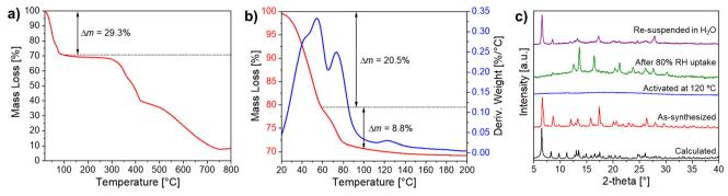
Fig. 2 Thermogravimetric and PXRD characterizations of Ni-ZW-MOF. a) Full TGA profile under N2 atmosphere ranging 20-800 °C; b) TGA (red) and DTG (blue) profiles in the <200 °C range; and c) PXRD analysis after different water adsorption and desorption processes.
