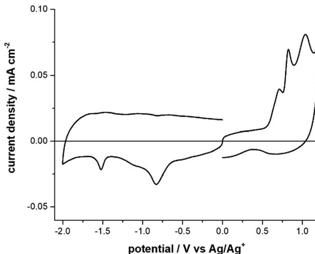
Fig. 2 Cyclic Voltammograms of **DTDPAB** molecule, in acetonitrile + 0.1 M Bu<sub>4</sub>NClO<sub>4</sub>. Scan rate: 0.1 V s<sup>-1</sup>.
